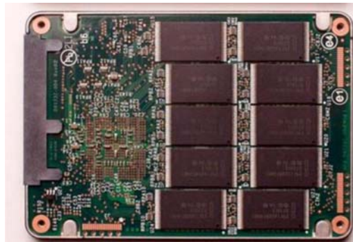
Figure 3. Flash Solid State Disk Inner Structure
